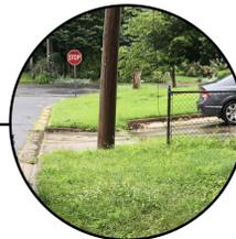
The potential sidewalk does not have adequate clearance to pass either in front or behind the existing utility pole.
