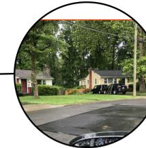
Large trees in front yards of #915 (left side photo) and #913 (right side of photo). The trees are 16" Red Maple, and 34" American Sycamore. The Sycamore appears to be in excellent condition. The critical root zone is estimated at 34 feet. Constructing the sidewalk at the back of existing curb would impact these roots significantly.
