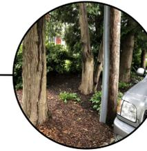
Existing utility pole and cluster of trees (American Arborvitae) near the curb in front of #911. These trees would have to be removed if the sidewalk were to be built behind existing curb. Moving the curb and sidewalk into the street would preserve these trees.
