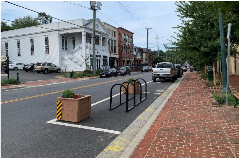
On-street bike parking corral on Church Street provides parking for up to eight bikes in place of one vehicle
