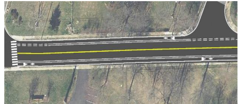
Figure 7-14: Shoulders to Bike Lanes on Courthouse Road
